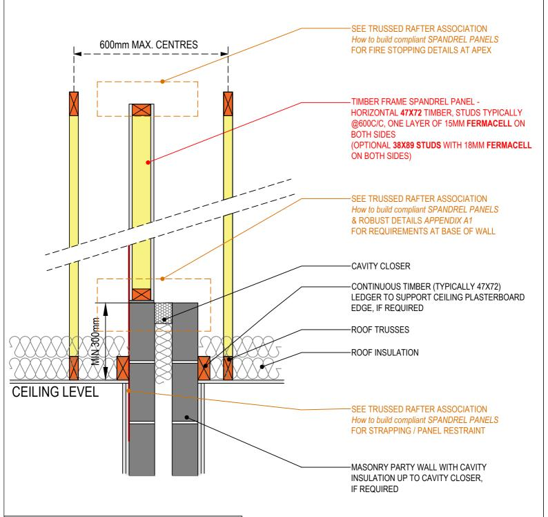
Timber Frame Spandrel Panel TYPE 1; for Masonry Wall (Single skin Fermacel **PANEL**
