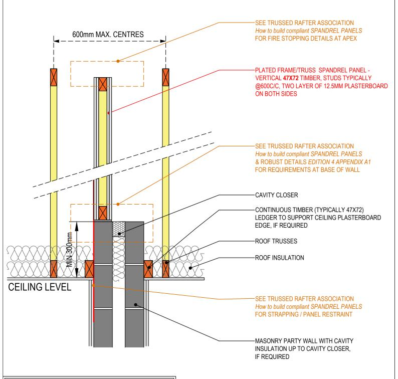
TYPE 2; Plated Spandrel Panel for Masonry Wall (Two layers of Plasterboard)
