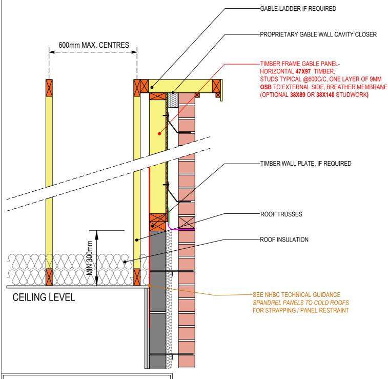
TYPE 4; Gable Panel for Masonry Wall
