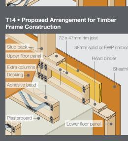
T15 • Proposed Arrangement for Timber Frame Construction
