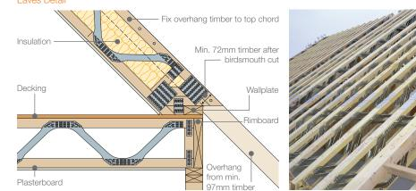
**Roof Bottom Chord Restraint Detail**
