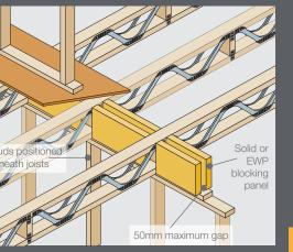
M8 • Parallel Restraint Bracing -Opening greater than 600m
