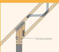
T12 • Top Chord Support with Double Rimboard T16 • General Arrangement for Timber Frame Construction per floor sole plate 72 x 47mm rim joist easi-ioists® tal Solid or composite top chord bearing timber rimboard Sheathing íΠυμ SYSTEM R4
