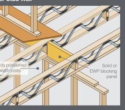
T4 • Intermediate Support (on to stud wall)
