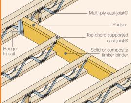
G5 • Intermediate Support (on to block wall)
