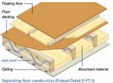
E-FT-3 Separating Floor – Metal Web Joists Use with Timber Frame walls only
